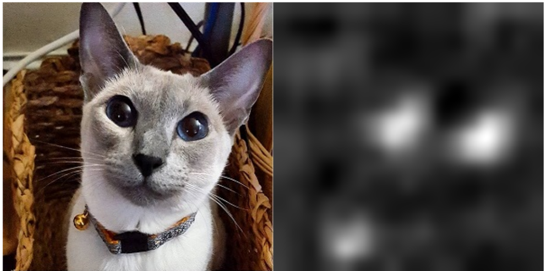
Figure 36: Strongly activating feature in fifth convolutional layer compared to the source image. We can't see the overall outline of the cat here, but can still identify what look to be the eyes and the bell.
